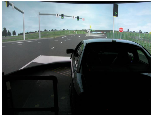
Figure 2. FHWA motion-base driving simulator.
